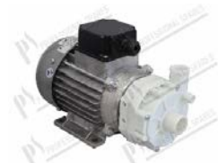
Wash pump 3 phase 110W 230/400V 50Hz 1,4/0,8A inlet Ø 28 mm; outlet Ø 26 mm
