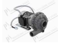
Wash pump 3 phase 900W 230/400V 50Hz 4/2,3A inlet Ø 63 mm; outlet Ø 48 mm; 2800 rpm; cable L=1050 mm
